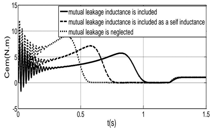
Fig. 8. Transient electromagnetic torque of DSIM.
