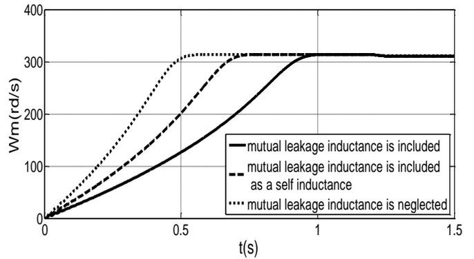
Fig. 7. Transient rotor speed characteristics.
