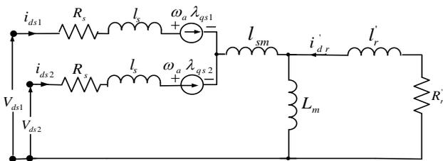
Fig. 2. d-axis equivalent circuit of a DSIM in arbitrary reference frame.
