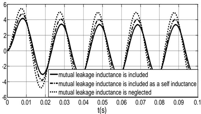
Fig. 10. Zoom of the time waveforms of current  $i_{s1}$  of the DSIM.
