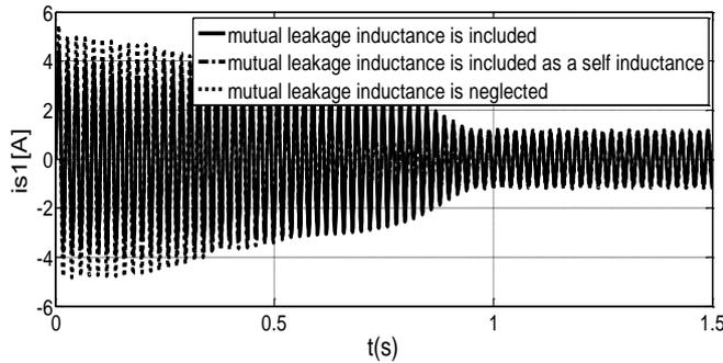
Fig. 9. The time waveforms of current  $i_{s1}$  of the DSIM.
