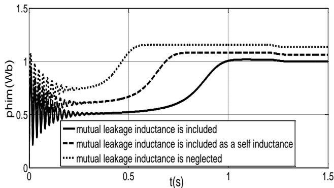
Fig. 11. Effect of the stator mutual leakage inductance on the magnetic flux.
