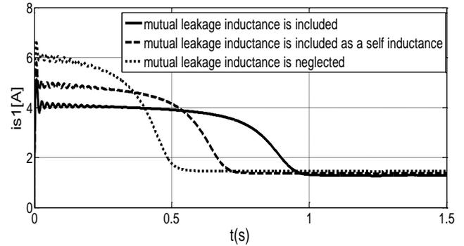
Fig. 12. Effect of the stator mutual leakage inductance on the stator current.
