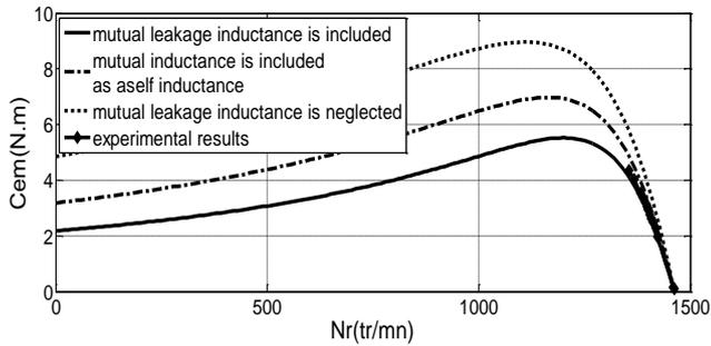
Fig. 3. Characteristic of the electromagnetic torque.
