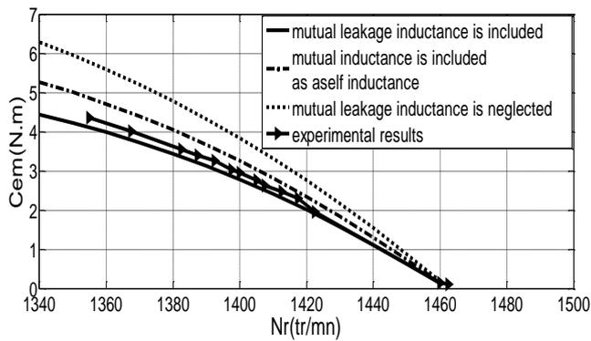
Fig. 4. Zoom characteristic of the electromagnetic torque with speed.
