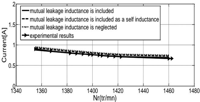
Fig. 6. Characteristic of current with speed.
